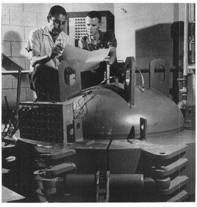
DISCUSSING specifications for a component inside large hydrostatic test vessel are Juan Mata, left, and Sam Martin. The tank can test items up to seven and one-half ft. long when filled with water under pressure. It is used for structural and leak testing.
